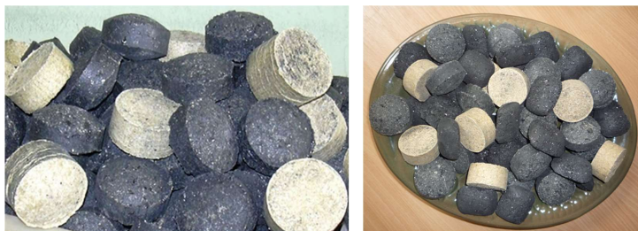
Fig. 1. Samples of fuel briquettes made in laboratory and industrial conditions
